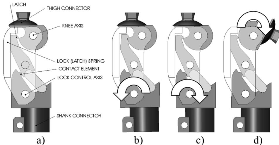
Fig. 2. (a) Prototype knee. (b) Lock engaged as a result of lock (latch) spring and/or flexion moment created at the control axis. (c) Lock disengaged due to extension moment generated at the control axis. (d) Knee joint shown flexed due to a flexion moment at the main knee axis.
