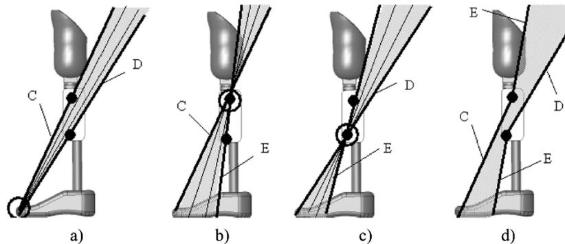
Fig. 3. Knee stability analysis for a knee joint with two stability-affecting axes. Boundary load line vector represented as thick line and other instability creating load line vectors as thinner lines. Shaded area represents all the possible instability causing load line vectors. (a) Vectors originating from toe-load boundary (labeled C and D). (b) About main knee axis (labeled C and E). (c) About the control axis (labeled D and E). (d) Overall zone of instability.
