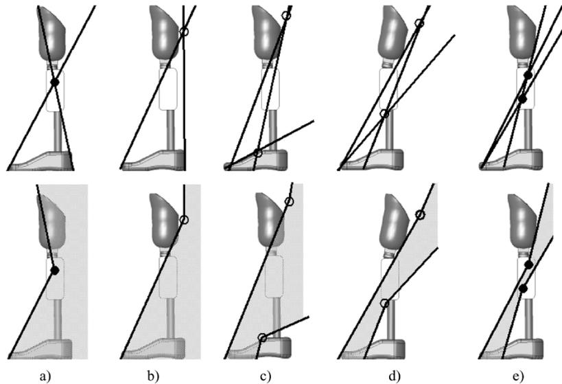
Fig. 4. Top diagrams show the boundary load lines for each knee and bottom diagrams the resultant zones of instability. Knee joints depicted are: (a) single-axis; (b) four-bar knee; (c) six-bar knee; (d) six-bar knee during stance-flexion; and (e) prototype knee. Axes that are instantaneous centers are shown as hollow circles and physical or fixed axes are solid circles.
