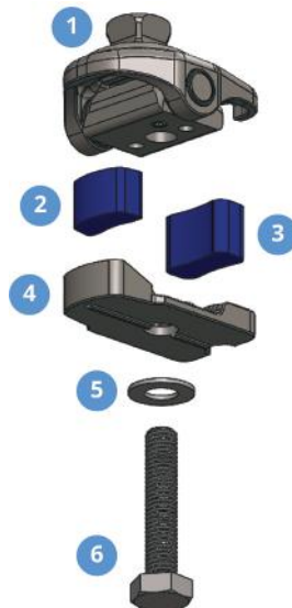
Fig. 8 Adjustable Stance Flexion Adaptor Assembly
