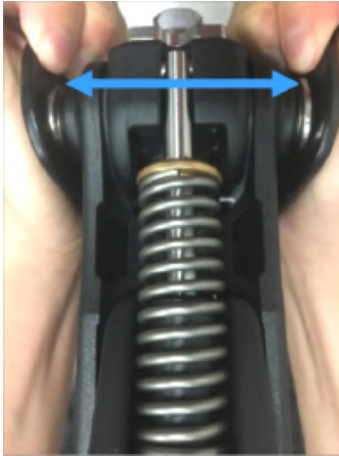
Fig. 20 ATK HydraPro Cover Removal
