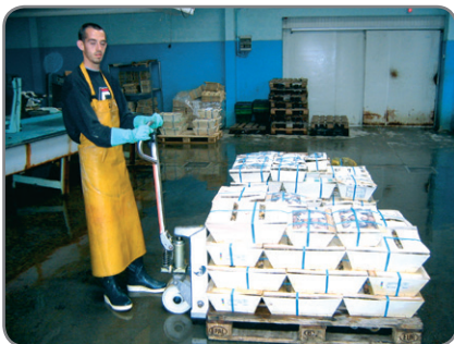
Inox - for the food industry in areas, where hygiene demands are not so high, but corrosion resistance important.
