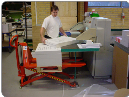
The manual highlifter needs very low power for the pump function and has foot protection and neutral position.
