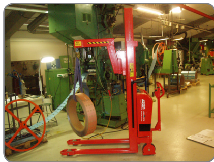
The crane arm in the component industry.
