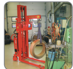
Metallic reels are lifted into a punching machine.
