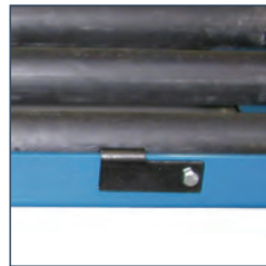
FLIP-UP BATTERY SAFETY STOP
