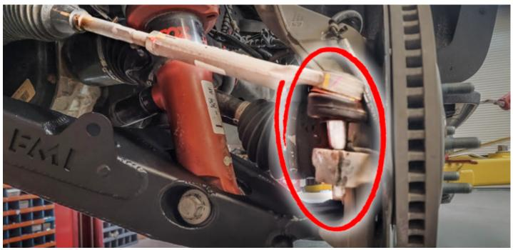
With a hammer -Strike the spindle where the tie rod went through to get it to dislodge.
