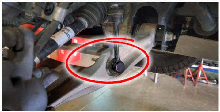
This allows the lower control arm to pivot down for more room to get the shock out
