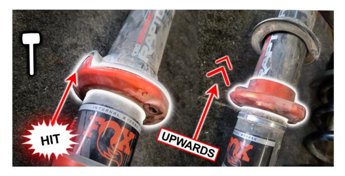
After the spring perch has been dislodged, make sure to have the small keepers stay on the shock - the collar will sit on this.
