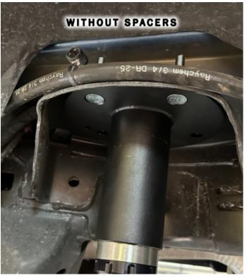
If you are adding a rear spacer plate, now is the time to install that with the supplied bolts, it installs onto the new bump stop.
