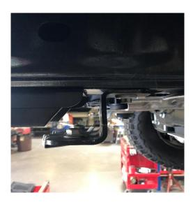
3. Remove rubber/plastic ring that is on the stock bumper where the tow hooks are. Careful as there are clips attached.
