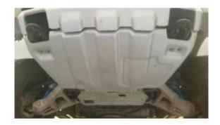
2. Remove the single bolt in skid plate front support bracket in the picture. Again, save the bolt as you will re-install this near the end of the project.
