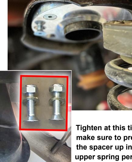
Tighten at this time, make sure to press the spacer up into the upper spring perch as you tighten so that the spacer sits flush in the spring perch.
