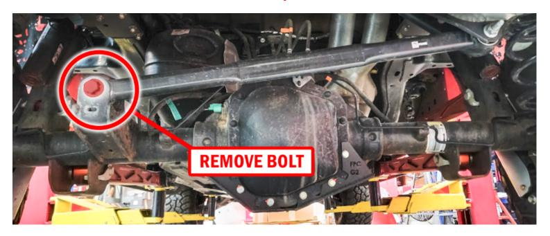
• Then lift the truck by rear diff and set on jack stands by the frame so suspension can fully droop and the axle can hang by the shocks
