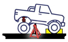
Alternatively, you can lift the truck off of the hitch until the rear tires come off the ground, then support the vehicle with stands.
