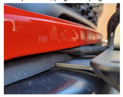
Before bolting the bumper down tight, make sure it's lined up and Matches the body lines, then torque to factory spec.
