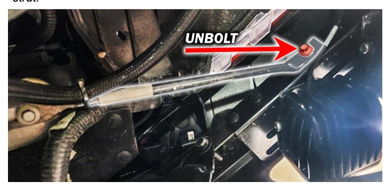
Unbolt this from the bumper and loosen at the frame side so that it can be rotated out of the way.
