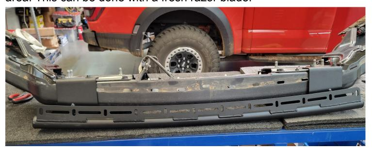
Repeat the same process for the rubber trim strip on the other side. Test fit as necessary, then once done, reinstall. This can be done by pressing down over the smaller clips, and the white clips press back through the black retainer to secure it to the bumper.
