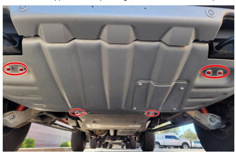
Remove the front skid plate by removing the two bolts on either side by the tow hook, and then the 2 bolts at the bottom of the skid plate by the lower control arm mounts.
