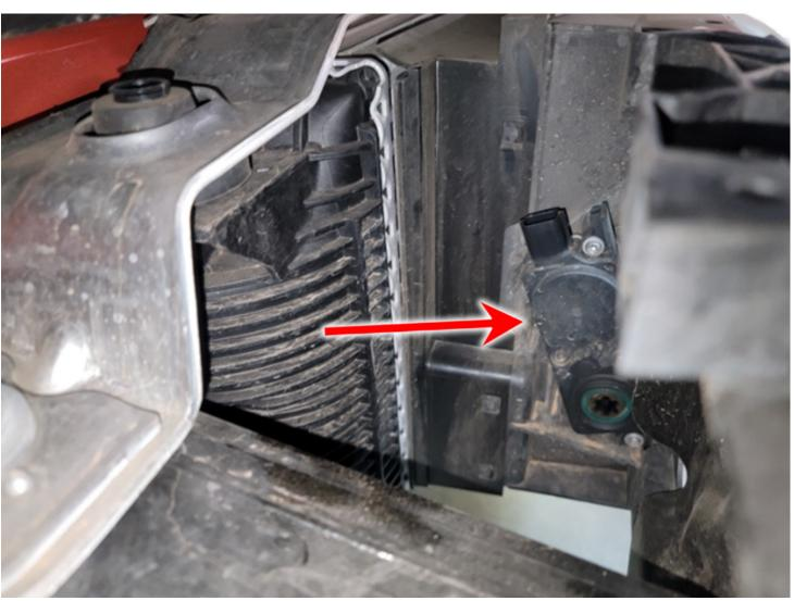
On the inboard side of the actuator is a plug, unplug this by pressing down on the release latch and pulling the plug up.
