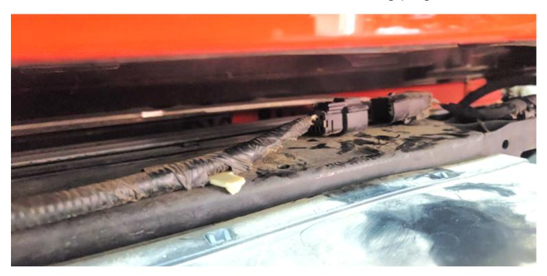
The two wire loom plugs can be removed with a panel tool, and the electrical plug can be undone by pressing down on the release latch and pulling the plug out.
