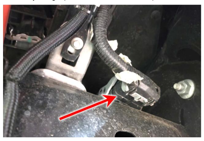
Once the plug is off the frame, there is a release tab that holds the gray lever down. Press the release tab while lifting up on the gray handle. After the handle is straight up, the plug can be undone. To plug it back in, reverse order making sure that the plug is properly aligned
