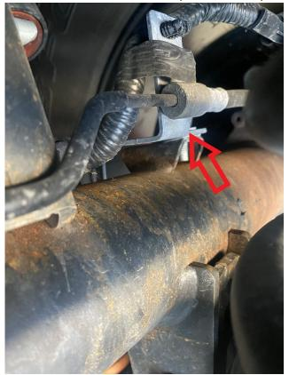
Route wiring under bump pad, between Axle Strap and Bump Pad. Secure Brake Line and wiring with zip ties. Install Axle Strap to Bump Stop Strike Plate with supplied hardware and tighten. Torque upper link bolt.
