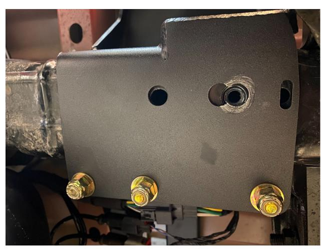
**3.** Place Bump Stop Mount Inner Support in frame. Align holes with Bump Stop Mount, and install and tighten (6) bolts. Tighten factory bump stop bolt. Repeat on other sides. On the passenger side, the exhaust section removed earlier provides room to get the Inner Support into position.
