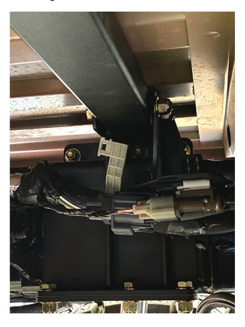
**5.** Remove the nut from the upper suspension link. **DO NOT REMOVE BOLT.** Remove Plastic wiring support from upper control arm mount. Place Bump Stop Strike Pad onto bolt, and reinstall factory nut. Trim Plastic wiring support to clear bump pad, and reinstall clips.
