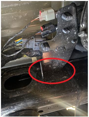
**5.** Before continuing with installation, inspect frame rails in the areas where the bump stop brackets will be installed for excessive weld build up. Grind smooth any protruding weld areas. Paint any bare metal areas.
