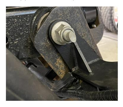
Grind friction weld holding mounting tab off brake flex line to remove mounting tab, and route between Axle Strap and Bump Pad.
