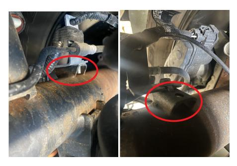
**4.** Remove wiring from frame mount on the driver side frame rail, behind the fuel tank. Cut off and grind smooth. Paint any bare metal.
