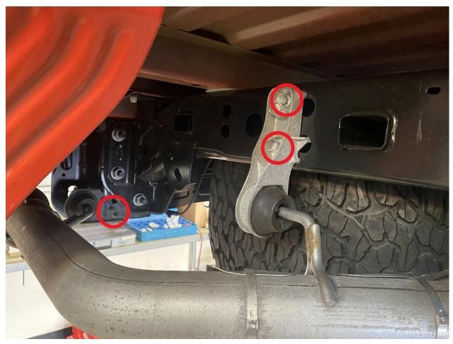
**3.** Remove brake line hold downs and wiring from axle mounts, outboard of upper link mounts. Cut off and grind smooth. Paint any bare metal.
