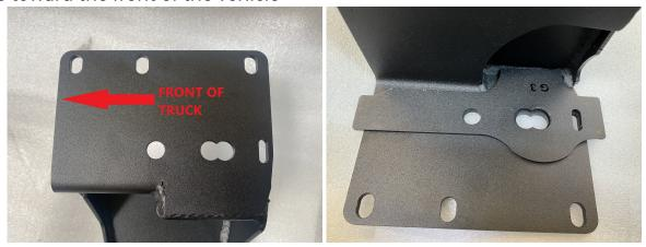
2. With the Lower Frame Spacer aligned with the Bump Stop Mount, as shown above, hold both up to frame, align single hole with unthreaded hole in frame, and the rear "figure 8" hole with the threaded factory bumpstop hole. Loosely install factory bump stop bolt to hold Bump Stop Bracket on frame. Repeat on other side.
