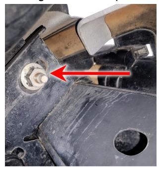
Then remove the two nuts on the front of the bumper on each side.
