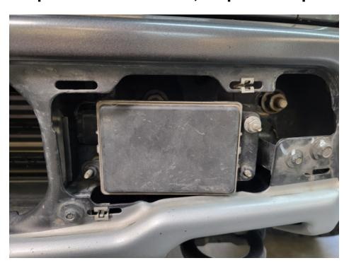
Then unplug the module, set aside for reassembly
