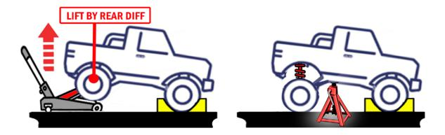
Alternatively, you can lift the truck off of the hitch until the rear tires come off the ground, then support the vehicle with stands. **DO NOT work under an unsupported vehicle.**
