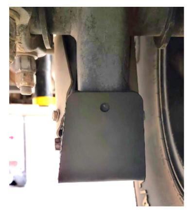
the drilled hole and tighten. Install the bolt from the outside of the skid inward, so that the nut is on the inside of the lower shock mount.
