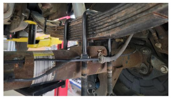
Once removed, loosen the u-bolts enough that the axle strike pad can be put in between the leaf spring pack and the spring perch on the axle. Make sure the strike pad goes around the center pins as you retighten the u-bolts.
