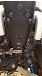
9. Slide the tow hook over the rear bolt in the middle of the "sled" and put front stock bolt back in, thread in but do not tighten.
