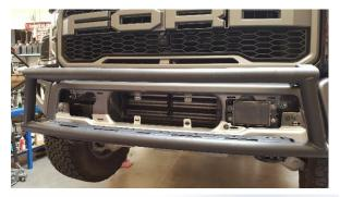
14. Locate the upper strut sections. You will notice one right and one left that are cut differently to match the contour of the factory bumper.
