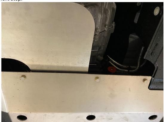
**4.** Using (2) supplied 10mm bolts, align Front Skid Plate, Center Skid Plate, and both Spacer Plates. The Spacer Plates are directional, and care should be taken to ensure all holes are properly aligned before proceeding. The correct order of assembly, from bottom to top is - Front Skid Plate, Center Skid Plate, (2) Spacer Plates
