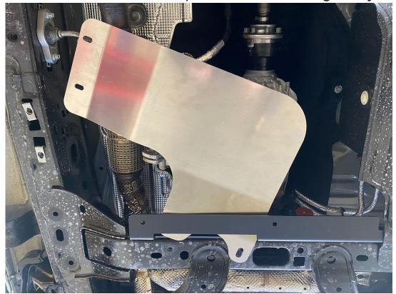
**3.** Hold Center Skid Plate in position. Install and finger tighten (3) included  $\frac{3}{8}$ " bolts and (3)  $\frac{3}{8}$ " nuts through the Rear Crossmember with washers on each side. Allow the front of Center Skid Plate to hang down for the next step.
