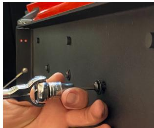
The included spacers are Used on the top 3 bolts, The bottom 2 bolts do not Need spacers
