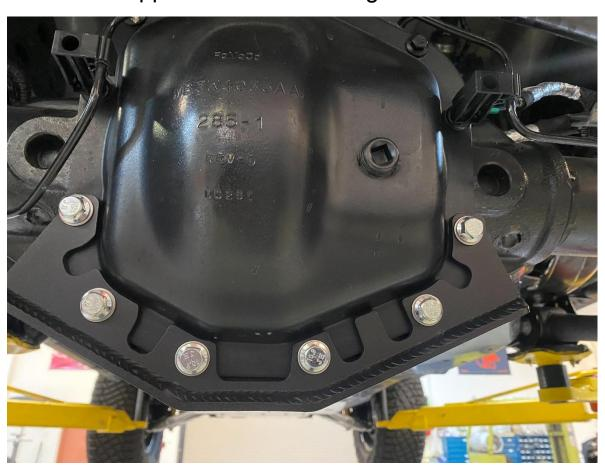
Ram TRX or Raptor & Bronco with Ford Performance Cover: It is required to have spacer washers between the diff skid and the cover. Use supplied M8 bolts and tighten.
