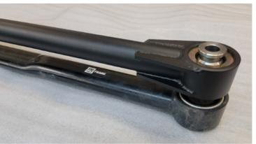
If a lift is installed: adjustment of the bar to make it longer will be required. Adjust it now to the calculated value and reinstall.
