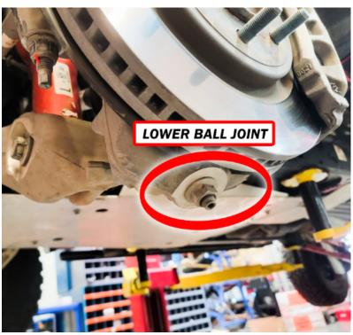
Then strike spindle next to each ball joint to remove the upper ball joint nut and Tie rod nut.
