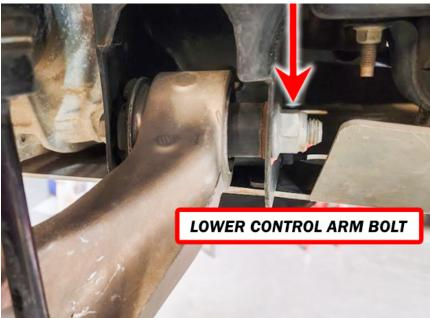
Step 9: Install new lower control arm with stock lower control arm bolts
