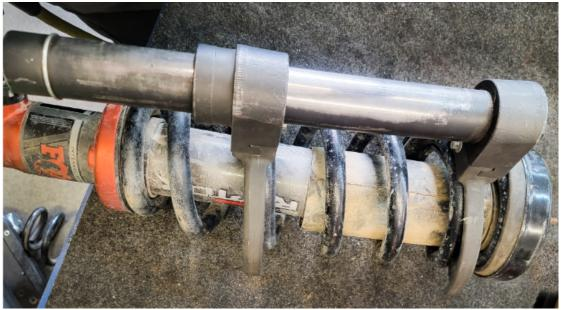
Once spring is compressed and under tension remove the top of the shock nut.
