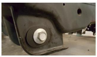
12. After you drive the truck for abour 100 miles, you should re-check the torque on these bolts.
