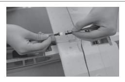
3 Connect the aileron servos with Y wires.
