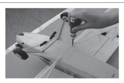
Fix the wing struts and landing gear with PWA 2\*10mm screw.
