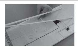
7 Install wing struts as shown.
