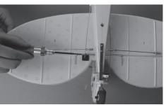
Insert the pushrod into elevator quick -controller and tighten the screw(the servo should be in center position).
