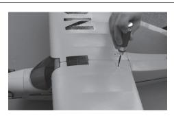
Fix the wing on fuselage with PA2.3\*20mm screw.
