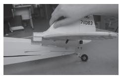
**9** Insert the horizontal stabilizer and vertical stabilizer in place.
