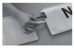
**1** Push Φ8\*360mm fiberglass tube into the hole of wing, glue the left and right wings together.
