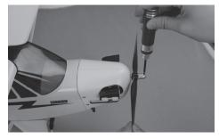
15 Install the propeller.
