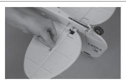
12 Install the horizontal stabilizer struts as shown.
