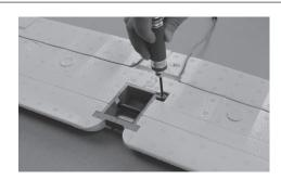
**2** Fix the wing with PA 2.5\*8mm screw.
