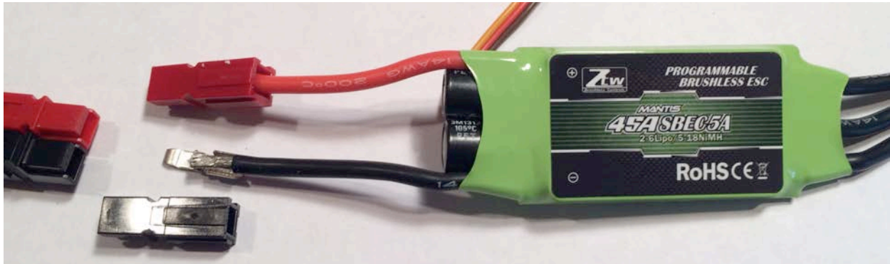
Figure 3 Powerpoles are being used to connect the output from the battery to the input of the ESC.
