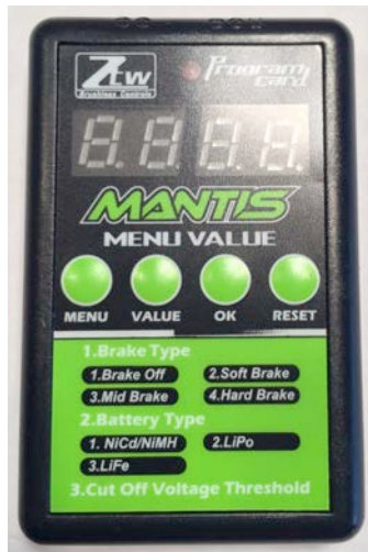
Figure 5 This programming card makes the task of programming the ESC much simpler and more precise.
