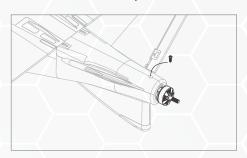
4. Install both fins for the V-tail. Be sure the screws that hold the plastic part of the hinge are looking up
