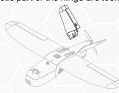
6. Install the battery hatch
