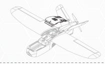
7. Lock the battery hatch twisting the peg
