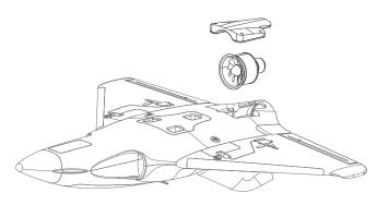
The EDF unit can be accessed through the dedicated hatch. Always firmly secure that hatch with the provided screws.
