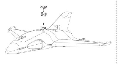
Install your FPV camera of choice on top of the 180° pan servo.
