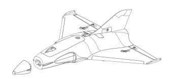
The nose cone is attached by magnets, providing a quick release, avoiding damage during hard landings.
