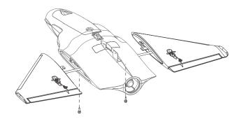
Install the main spar. Attach the wings and secure them with the provided thumbscrews
