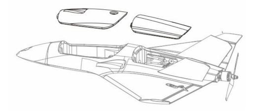
Once you placed all your FPV gear, be sure both hatches fit flushed against the fuse.
