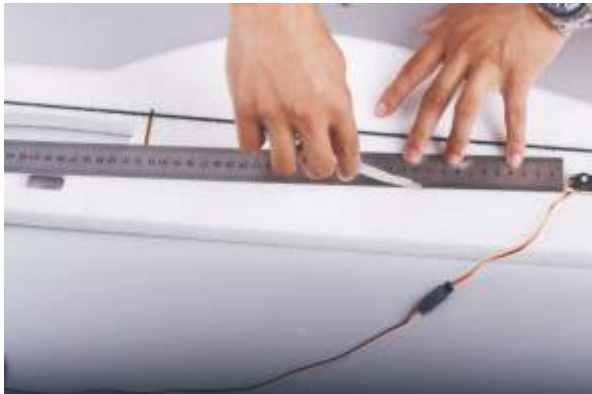
5. Use the hobby knife to cut a 10mm depth slot , make sure the servo wire to reach the receiver location .
