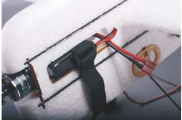
39. Install the lipo battery pack ,and then fix them with velcro.
