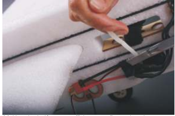
38. Use the knife to cut off the superfluous band .
