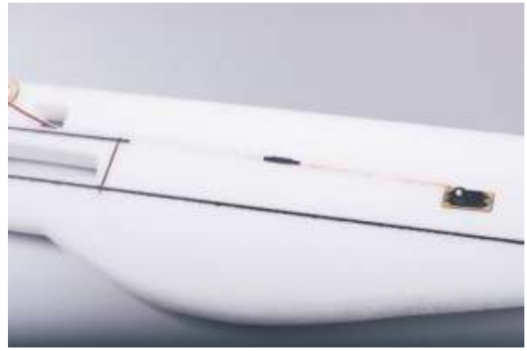
7. Use the same method to install the elevator servo as installing the rudder servo .
