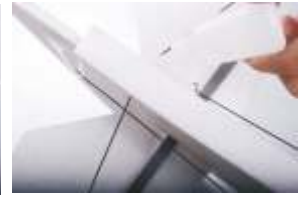
31. Glue 2pcs of 1.3mm*190mm carbon rods onto the back of the horizontal stabilizer and the both sides of the under of the fuselage. To avoid the twisting of the horizontal stabilizer.
