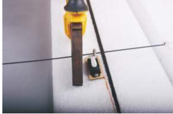
15. Use the pinchers to cut off the superfluous steel wire.
