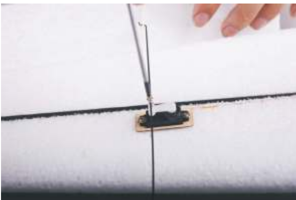
14. Install the Z-Bend , tighten the screws by using the screwdriver.
