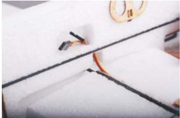
18. Thread the servo wire through the hole till the receiver location.
