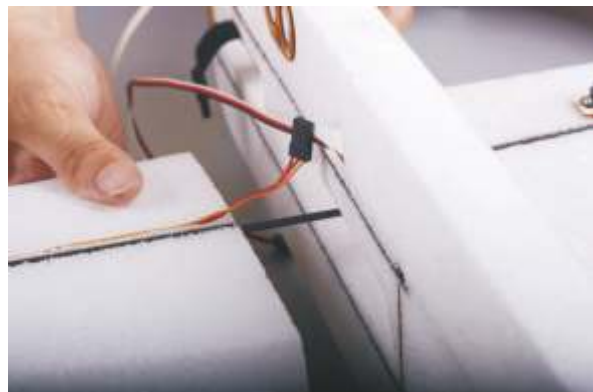
17. Connect the left and right wing with 3 x 100 mm carbon rod , insert it into the wing slot.
