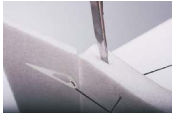
32. Use a knife to cut a slot under the fuselage.
