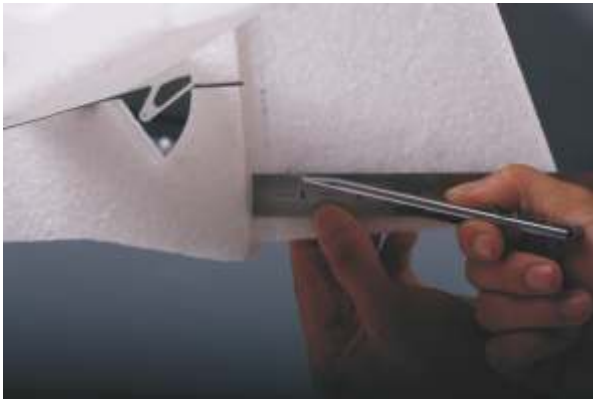
25. Use a knife to cut a hole into the rudder .
