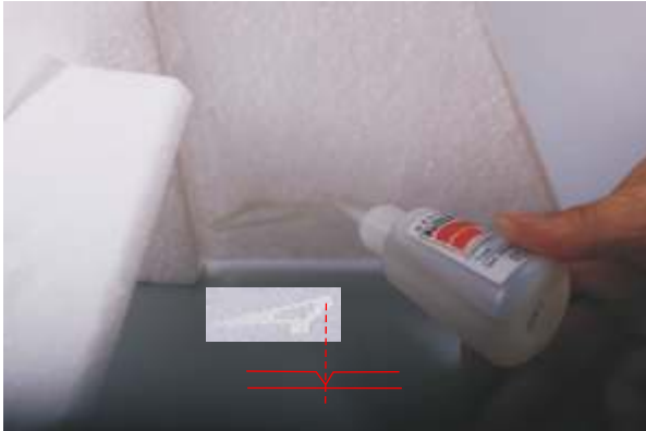
26. Glue the control horn by using CA .
