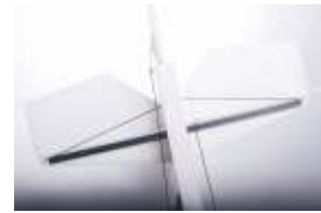
31. Glue 2pcs of 1.3mm*190mm carbon rods onto the back of the horizontal stabilizer and the both sides of the under of the fuselage. To avoid the twisting of the horizontal stabilizer.
