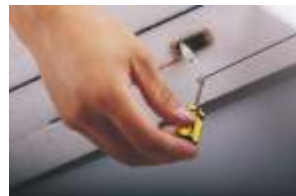
29. Install the Z wire onto the pushrod connector , and then tighten the screw with screwdriver.
