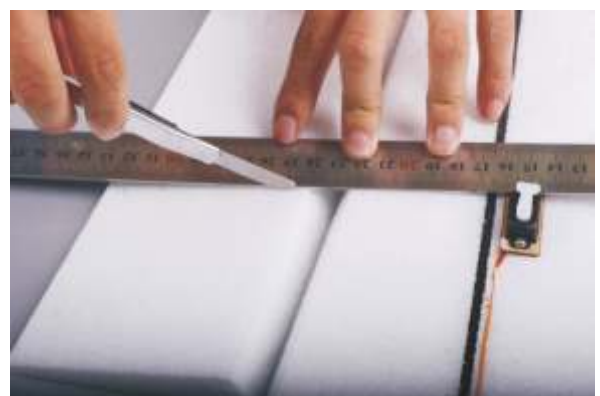
10. Pls use a hobby knife to cut a slot which is vertical to the servo arm , so that can install the servo control horn easily .
