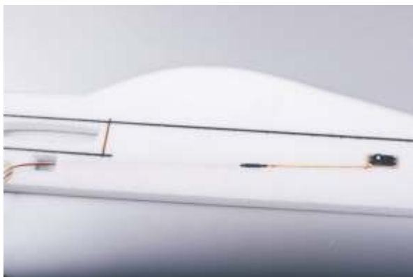
6. As the picture shown , insert the servo wire into the pre-cut slot .
