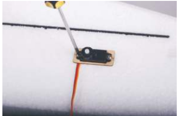
3. Fix the servo onto the servo arm by using 2pcs screw Pls pay more attention the servo wires when you fix the servo .
