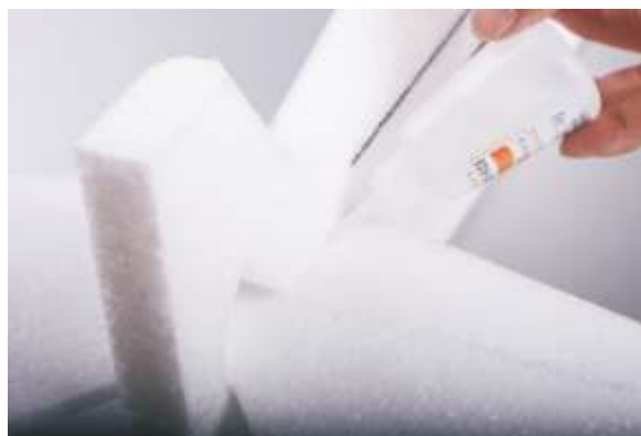
21. Insert the horizontal stabilizer into the fuselage slot using CA glue.
