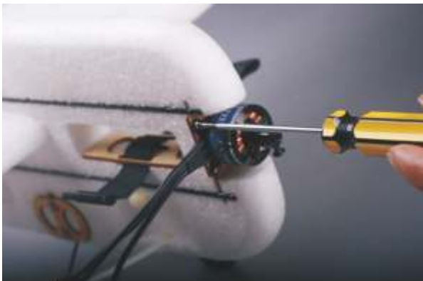
36. Install the motor into the motor mount ,and then tighten them by using 4pcs screws.
