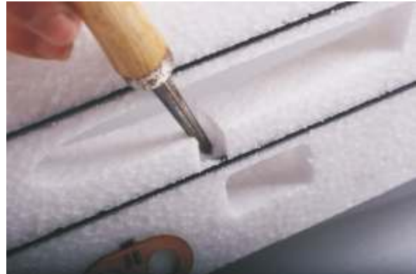
16. At the junction of the receiver and wing location ,cut a hole , convenient for the aileron servo wire pass through easily .
