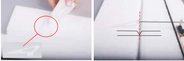
11. Glue the control horn by using the CA .
