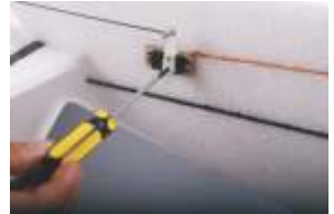
30. Center the rudder and elevator , and then tighten the servo arm .
