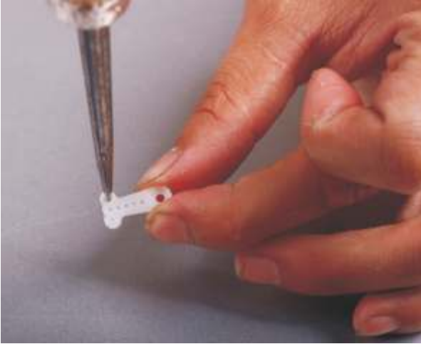
12. Increase the servo arm hole by using the aiguille , convenient for installing the pushrod connector.
