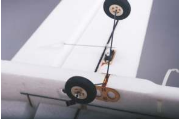
35. Insert the landing gear into the slot .
