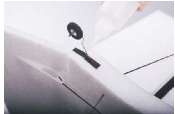
33. Glue the tail wheel set into the fuselage slot.
