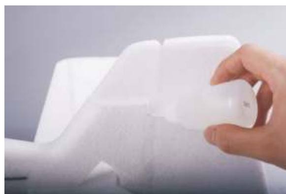
24. Glue the vertical stabilizer onto the fuselage.
