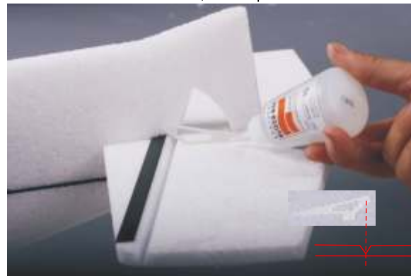
23. Glue the control horn using CA .
