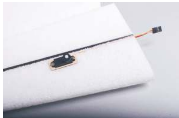
9. Use the same method to install the right aileron servo.
