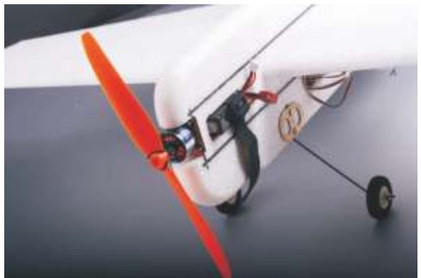
41. Fix the propeller with O-ring .
