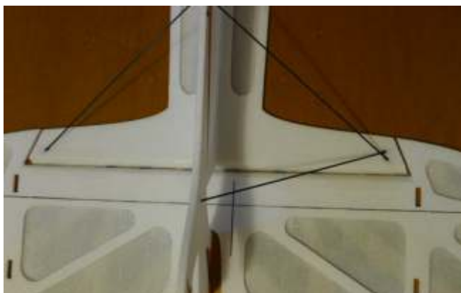
16. Install the 1 mm x 12,5 cm carbon rod.
