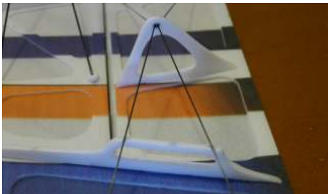
15. Fix with C/A the 0,8 mm carbon rods to reinforce the ailerons.
