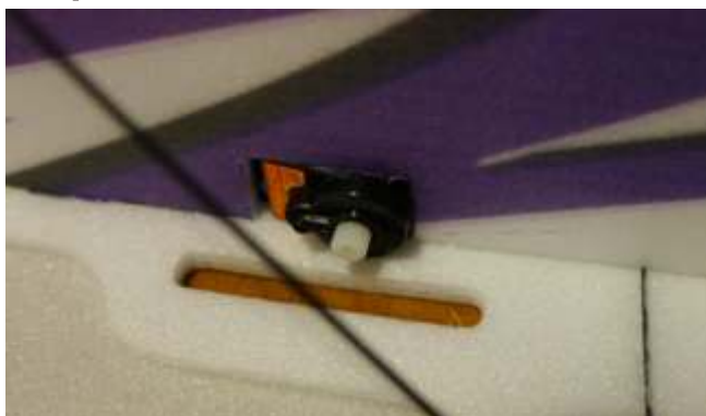
19. Use some C/A to fix the elevator servo in the pre-reserved slot on the lower vertical fuselage as shown in the picture.
