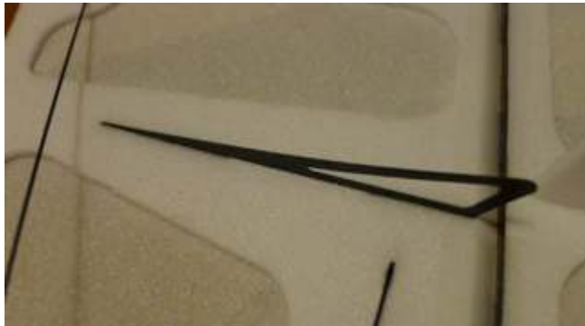
21. Fix with C/A the two ailerons control horns.
