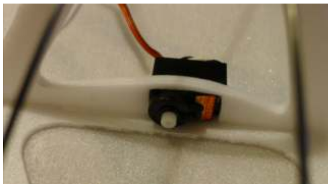
18. Use some C/A to fix the two aileron servos in the pre-reserved slots on the downside vertical winglets as shown in the picture.
