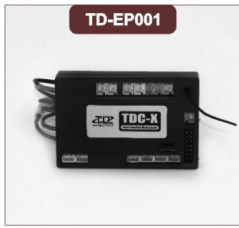
TDC-X功能主板(2.4GHz) TDC-X Multi-function circuit unit(2.4GHz)
