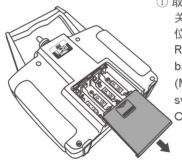
① 取下电池盖(开 关必须在OFF 位置)。 Remove the battery cover. (Make sure the switch is on OFF position.)
