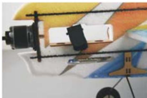
37. Connect motor and ESC, then adjust to correct motor running direction before flying. Put ESC into the slot of downside fuselage.
