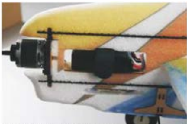
38. Insert battery into the battery hole.
