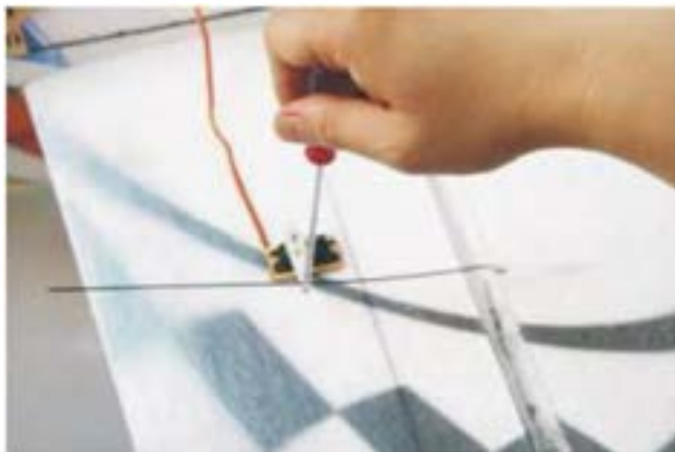
17. Use the screwdriver to tighten the pushrod connector with screws.
