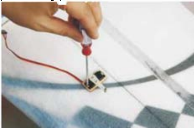
11. And fix the servos onto the plywood servo mount with included screws.
