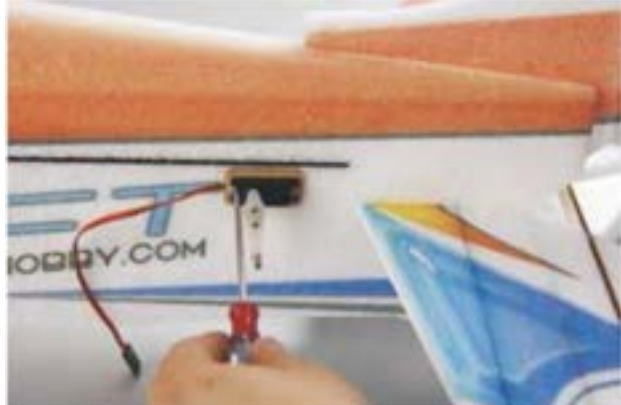
25. And fix the servos onto the plywood servo mount with included screws.
