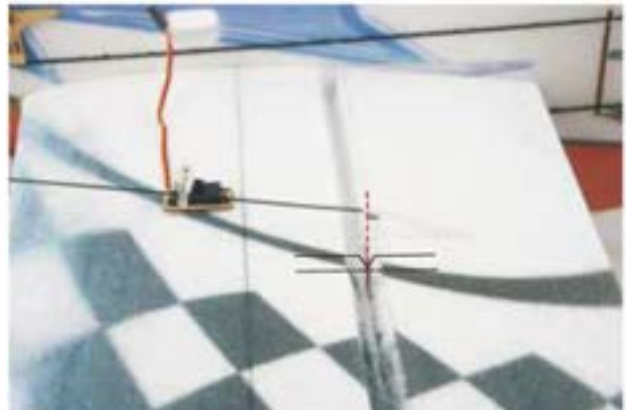
15. Through the other side of the Z bend to the hole of pushrod connector, and then insert the aileron horn into the pre-cut slot.
