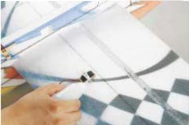
10. Put the servo into the pre-cut servo hole, then use glue to fix the servo mount onto the wing. Make sure the servo arm points to the wing tip.
