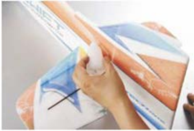
23. Use CA to fix the rudder.
