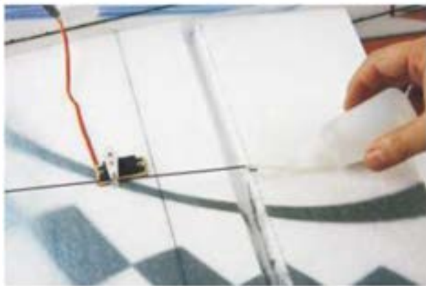
16. Glue the control horn by using the CA.
