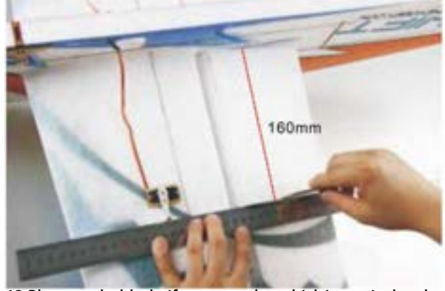
13. Pls use a hobby knife to cut a slot which is vertical to the servo arm, so that can install the servo control horn easily.
