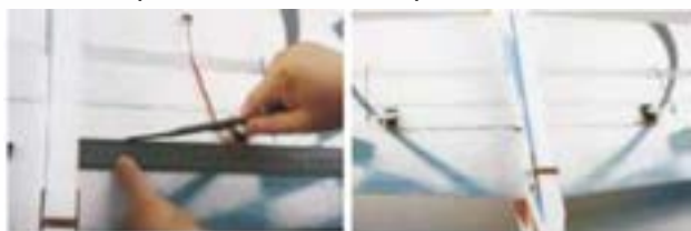
20. Use knife to cut slots on wing, then embed aileron servo leads as picture shown.
