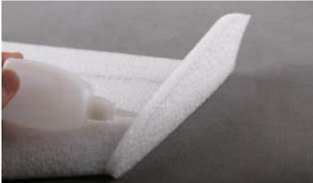
Install wing fences on wing tips with glue.
