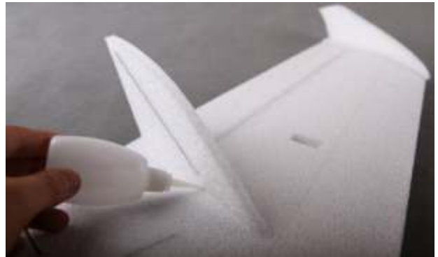
Insert rudder into pre-cut slot on wing and fix with glue.
