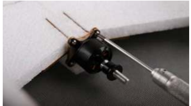
Fix motor on motor mount with mounting screws.
