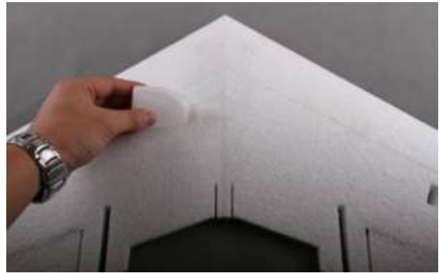
Glue left and right wings together.
