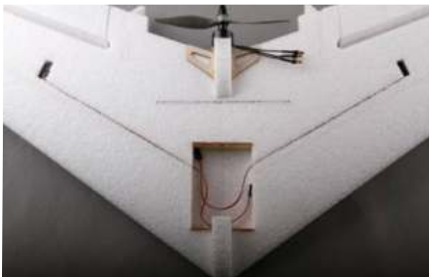
Embed the servo leads into slots.
