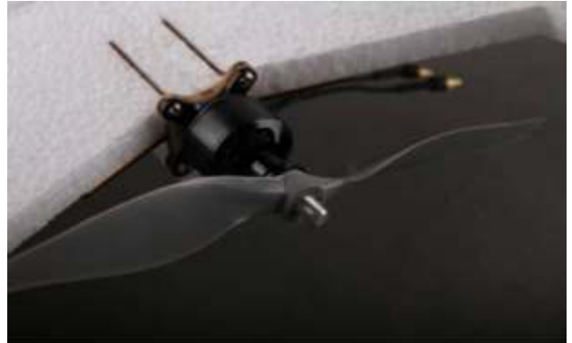
Fix motor on motor mount with mounting screws.
