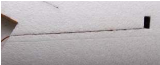
Then cut a slot on bottom wing for embedding the servo leads.
