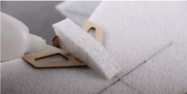
Fix another foam skid on bottom of motor mount with glue.
