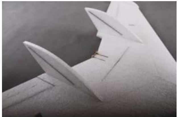
Insert rudder into pre-cut slot on wing and fix with glue.
