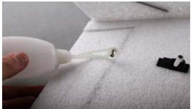
Install the control horn with glue.
