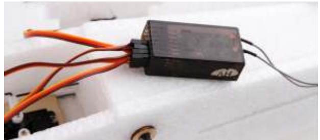
Insert all servo cables into receiver according to corresponding sequence.
