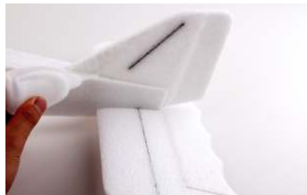
Put rudder tail on the end of fuselage, insert into the slots with glue, Make sure rudder and stabilizer is perpendicular to each other.
