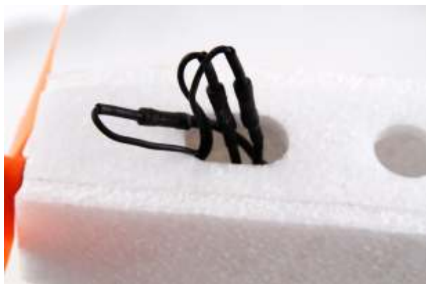
Connect motor cable to ESC cable
