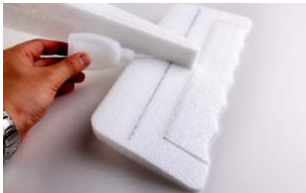
Put elevator tail on the end of fuselage, insert into the slots and fix the joints with glue.
