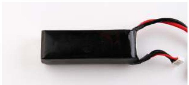
Battery:11.1V 3S 800—1800MAH
