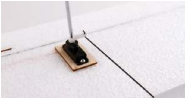
Lock screw on servo arm
