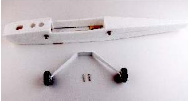
Fuselage,landing gear and the fixing screw.
