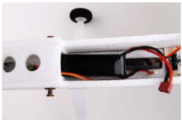
Battery:11.1V 3S 800—1800MAH Fix wing on fuselge by using rudder band
