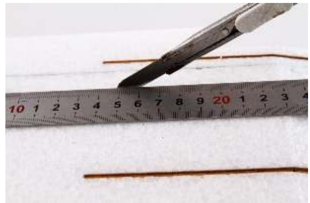
Cut the servo house by art knife
