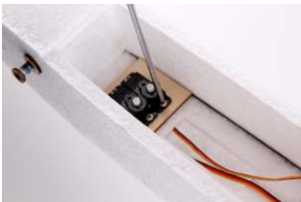
Fixing servo with screw
