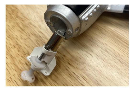
3) The motor and motor mount can now be pulled out of the fuselage.
