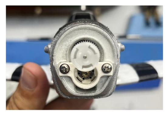
2) Remove the two screws that hold the motor mount in the fuselage.
