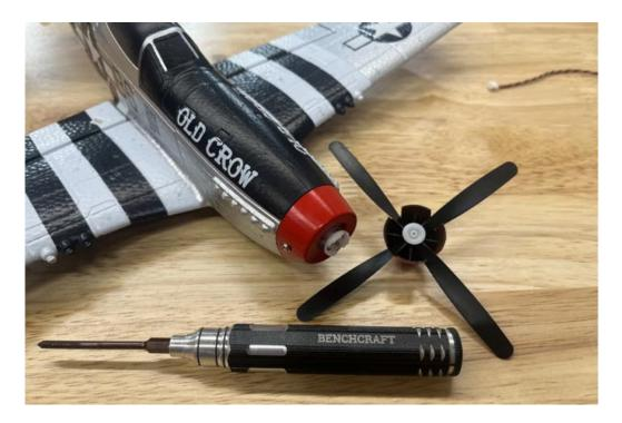
1) Remove the propeller by popping it off the motor. Then, remove the two screws that hold the cowling on.
