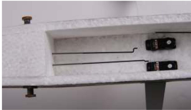
Elevator push rod 1.2*585MM Rudder push rod 1.2*585MM
