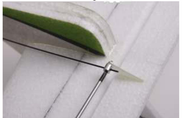
16. Plug the push rod into adjuster and keep the control surface in flat, then fix the adjuster with screwdriver.
