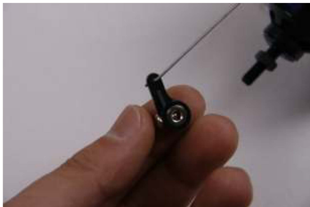
7. Connect the servo arm to Z bend.
