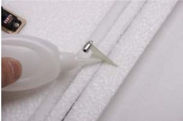
21. Cut a small slot on aileron for installing the control horn (position refer to above picture), then insert the control horn and fix with glue.
