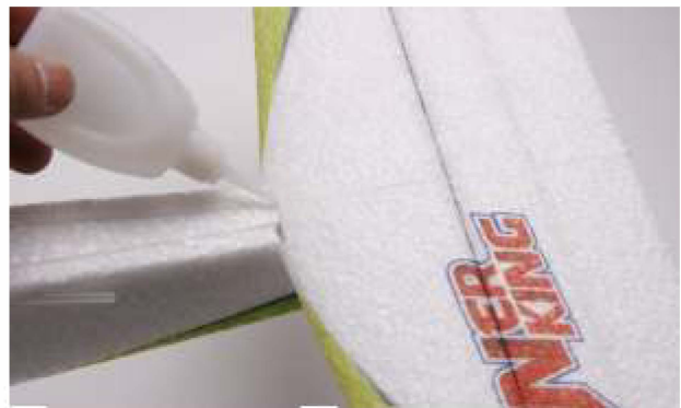
10. Install the stabilizer on the fuselage with glue.
