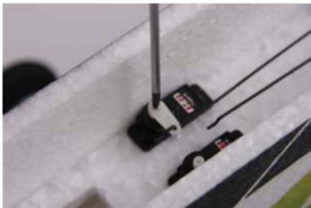
14. Connect the servo arm to Z bend, then use screw to fix the servo arm on servo.
