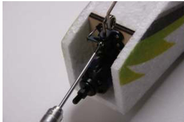
9. Insert the landing gear into corresponding place in above picture, then fix it with screw.
