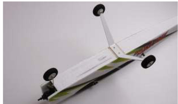
9. Insert the landing gear into corresponding place in above picture, then fix it with screw.
