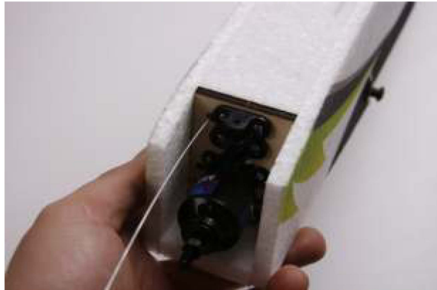
6. Insert the push rod (the end without Z bend) into the hole according to the position shown in the picture.
