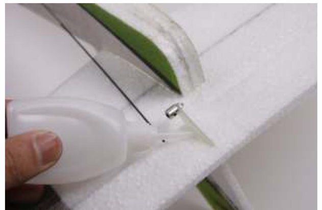
15. Cut a small slot for installing the control horn (position refer to above picture), then insert the control horn and fix with glue _ _ _
