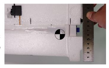
When using a battery other than the recommended Admiral 3s 2200mAh battery, always verify that the model balances at the recommended Center of Gravity (CG) position. Do not attempt to fly your model with a "tail heavy" CG position, which may result in loss of control and a crash.
