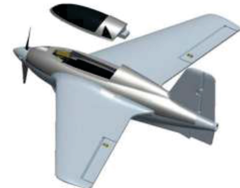
17. Power on and put battery inside equipment cabin, then cover the canopy.
