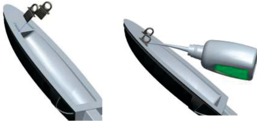
4. Install canopy clips in canopy, then fix with glue.
