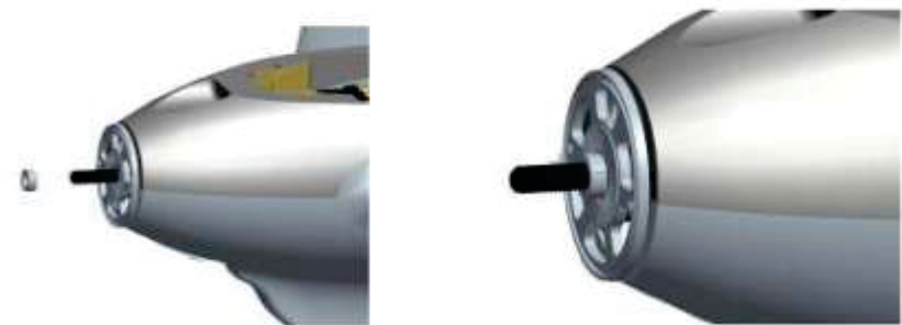
10. Put propeller hub on shaft.
