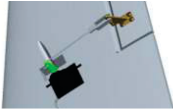
14. Install aileron push rod as pictures shown.
