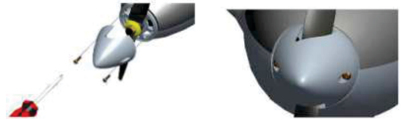
13. Install the spinner, then fix with screw.
