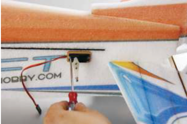
25. And fix the servos onto the plywood servo mount with included screws.
