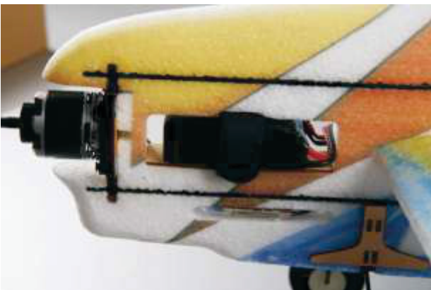
38. Insert battery into the battery hole.
