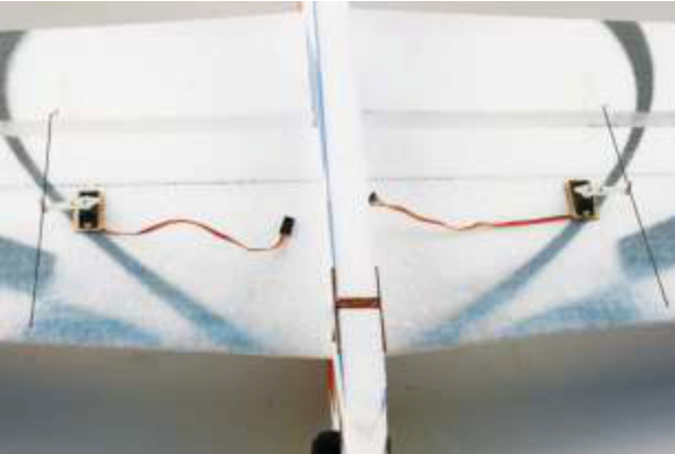
18. Use the same method to install the aileron pushrod.
