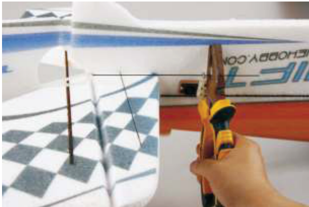
31. Use the pinchers to cut off the superfluous steel wire.
