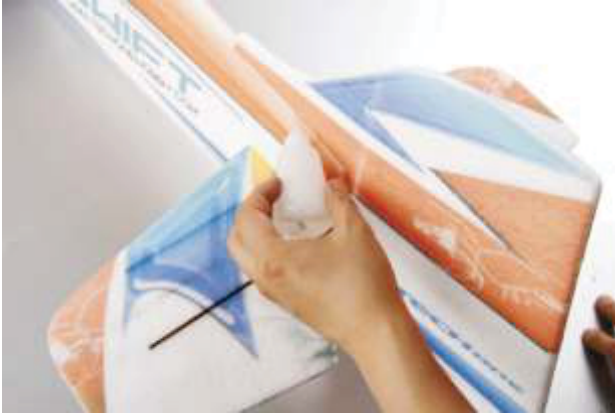
23. Use CA to fix the rudder.
