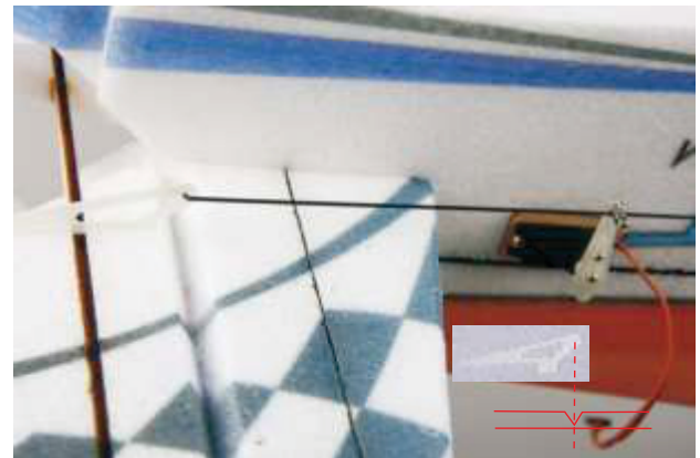
28. Through the other side of the Z bend to the hole of pushrod connector , and then insert the rudder and elevator horn into the pre-cut slot.
