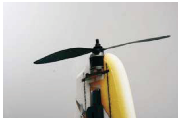
41. fix the propeller
