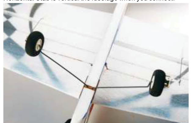
35. Insert the landing gear port into the slot of plywood mounting brace onto the bottom of the fuselage.
