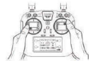
MODE1 (Japanese-hand gyroscope calibration)
