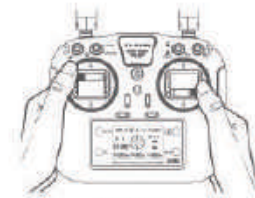
MODE2 (American-hand gyroscope calibration)
