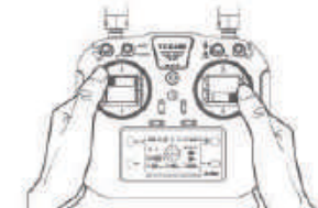
MODE1 (Japanese-hand gyroscope calibration)
