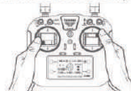
MODE2 (American-hand gyroscope calibration)
