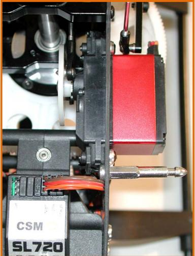
The cyclic servo wires are then fed inside the frames, along and down into the area underneath the front tail gearbox casing. The gyro wires were then fed down inside the right hand frame to join the cyclic servo wires on route. This chosen Spektrum 7600 receiver was fixed via velcro to the inside of the right hand side frame.
