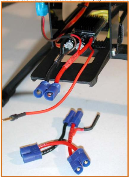
The Electronic Speed Controller (ESC) was mounted to the front of the lower base plate with velcro as shown below. The motor wires were then connected to the ESC and held out of harms way with a small velcro strap. The additional small red-wire is an anti-spark feature of the YGE 60 HV ESC. If you have ever connected a 12S Lipo, you will know just why this feature is included!
