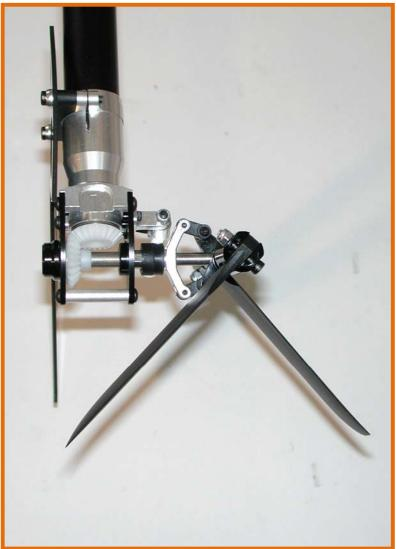
Now make sure that the lower folded back tail blade moves to this position when the rudder stick is moved to the left and when the nose of the helicopter is moved to the right.
