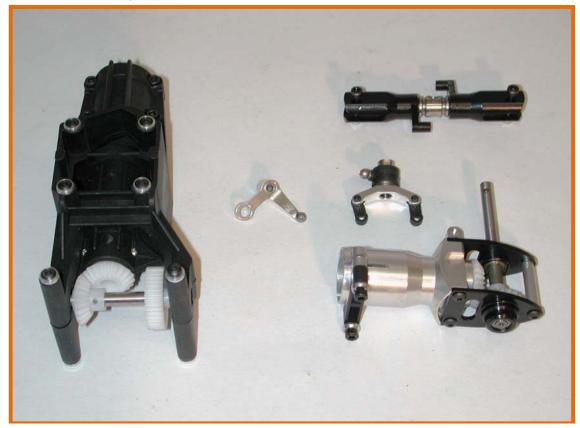
The tail rotor hub is now fitted to the tail shaft and locked in place with an M-4 set screw that seats in a recess in the shaft. I did check the threadlock on the tail blade grips and it was good, but it is always worth checking. The tail pitch assembly is then linked to the tail rotor grips via the control links and the tail rotor bellcrank is fixed in place. Be sure that everything operates smoothly before moving on.
