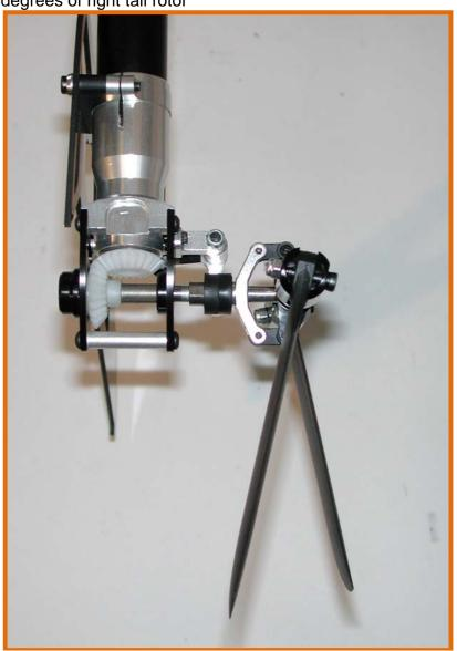
Now make sure that the lower folded back tail blade moves to the position below when the rudder stick is moved to the right. If the blades do not move to this position, then us the TX rudder 'Reverse' function and re-test. Now make sure that the lower folded back tail blade moves to the same position when the nose of the helicopter is moved to the left when the gyro is in 'Heading Lock' mode. If the
