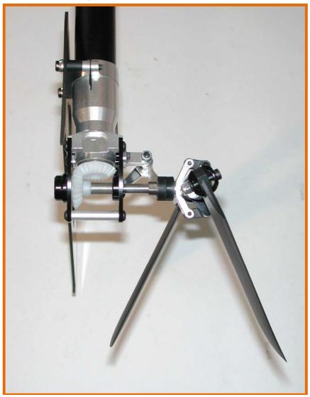
Finally, make sure that the tail servo is not binding or buzzing in any way at full left / right travels as this will damage the servo. If any binding is detected, reduce the gyro travel limits via the interface unit / dial as required.
