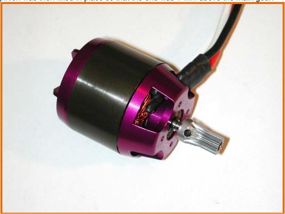
The motor was loosely positioned in place on the motor mount via 2 M-3 fixing bolts and steel washers. I then carefully slide the motor up to the main-gear so that
