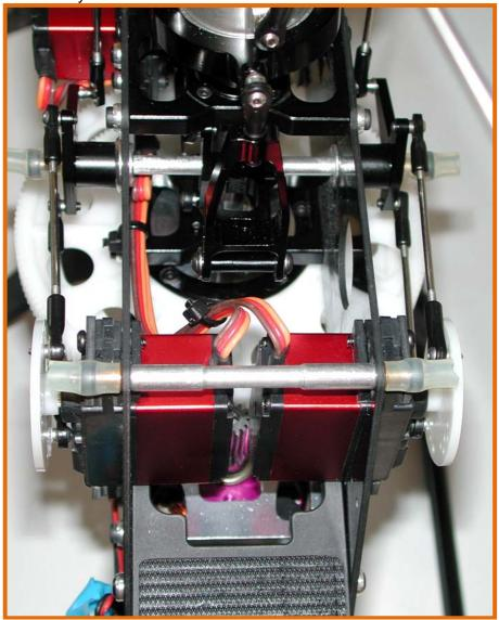
I did have to file the holes in the frames so that the rectangular servo fixing plates could be fitted to the inside of the frames. Also be aware that the rear elevator servo installation differs from that shown in the manual and should be mounted to
