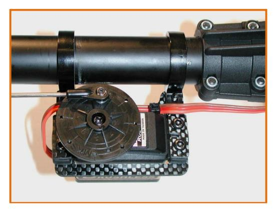
The next step is to link up the tail pushrod wire and adjust the length of the wire so that the tail blades have approx. 8 degrees of right tail pitch at servo neutral. Now straighten up the pushrod guides so that the tail linkage rod is a straight run when viewed down the end of the tail boom.
