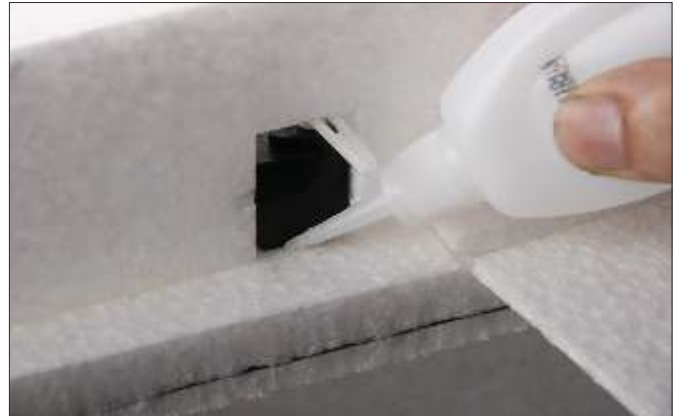
18. Fix the rudder servo into the pre-reserved servo hole with glue.
