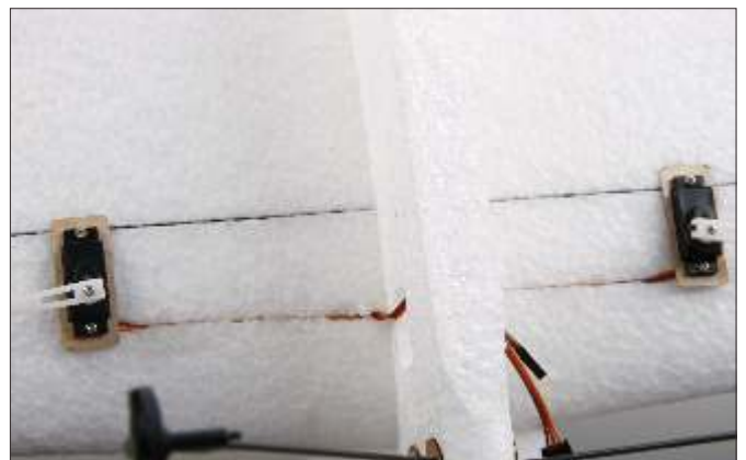
30. Use knife to cut slots on wing, then embed aileron servo leads as picture shown.
