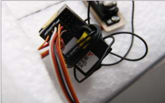
32. Link the servo leads and ESC to receiver, then test-fly.
