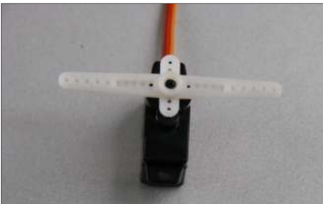
6. Put the servo into the servo hole, then use glue to fix the servo mount onto the wing. Make sure the servo arm point to the wingtip.
