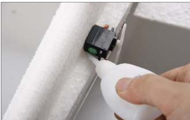
21. Insert the horn into the pre-reserved slot on elevator, then use glue to fix.
