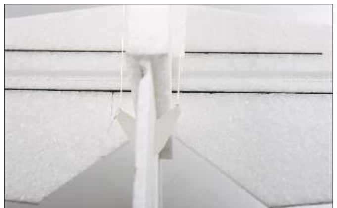
19. Insert the horn into the pre-reserved slot on rudder, then use glue to fix.
