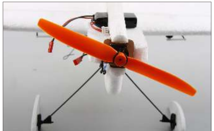
36. Use O-ring to fix the propeller .
