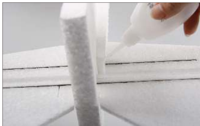
15. Drop some glue on the joints of elevator and fuselage to fix.
