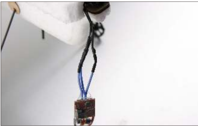
27. Connect motor and ESC, then adjust to correct motor running direction before flying.
