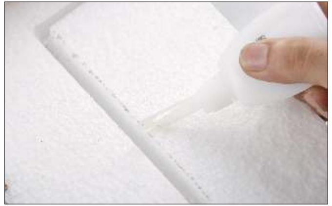
10. Fix the aileron horns with CA
