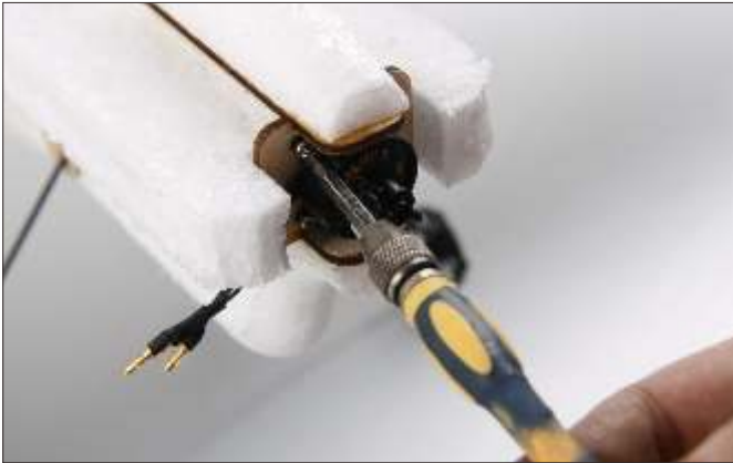
26. Use included screws to fix the motor onto the motor mount.
