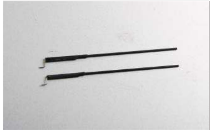
11. Cut shrink tube into 4pcs 20mm length, then use electric iron to install 2pcs Z bend and 2pcs carbon fiber tubes (size: 1.3*85mm), please refer to the picture.
