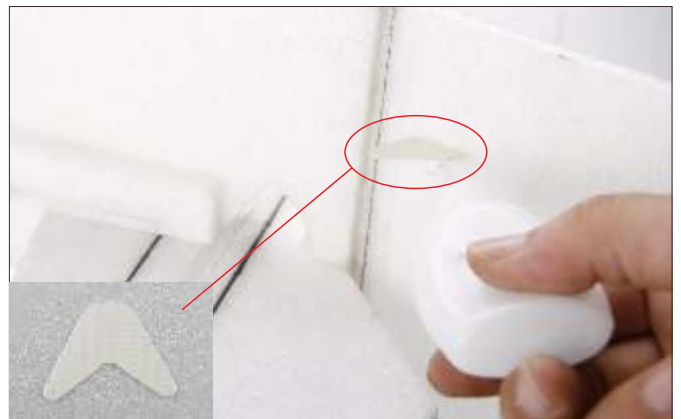
19. Insert the horn into the pre-reserved slot on rudder, then use glue to fix.
