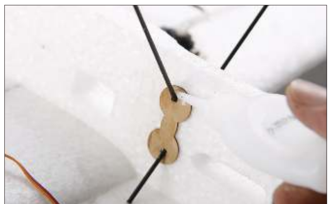
24. Push the landing gear through the plywood on fuselage and fuselage itself, then use CA to fix.
