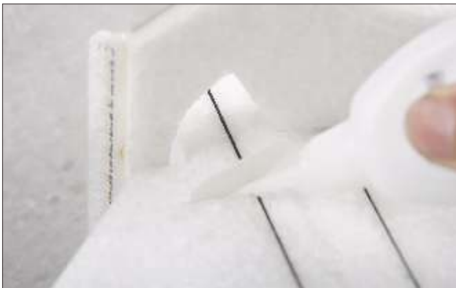
21. Insert the horn into the pre-reserved slot on elevator, then use glue to fix.
