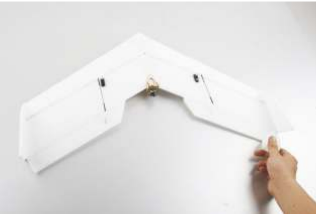
15. Glue the two wing fences by using CA.
