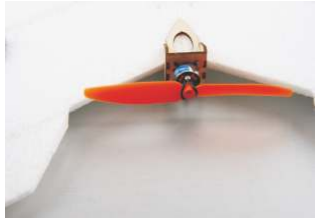
16. Fix the propeller by using O-ring.
