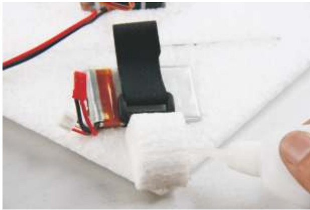
14. Glue the egg skid onto the nose of the flying wing , so that can prevent from damaging the Battery or receiver upon landing.
