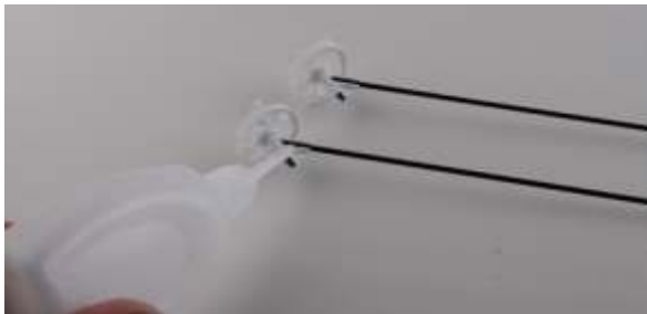
10. Insert 2*220mm carbon fiber rod into the slot on triangle part, then fix with glue
