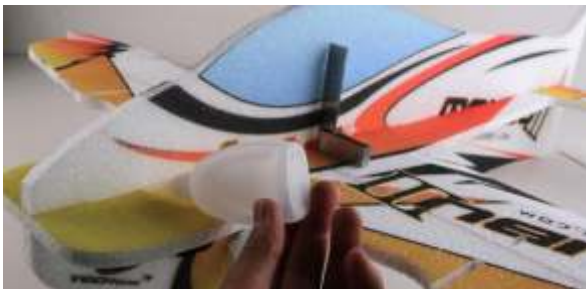
17. Insert upper fuselage into the slots on horizontal fuselage, then fix with glue Make sure the upper fuselage is perpendicular to horizontal fuselage,
