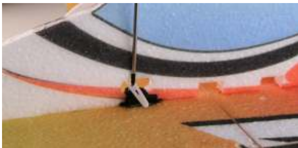
31. Install servo arm on servo and fix with screw
