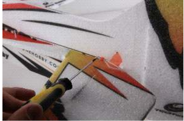
43. Adjust the plastic clip to the right place by screwdriver, then fix with screw
