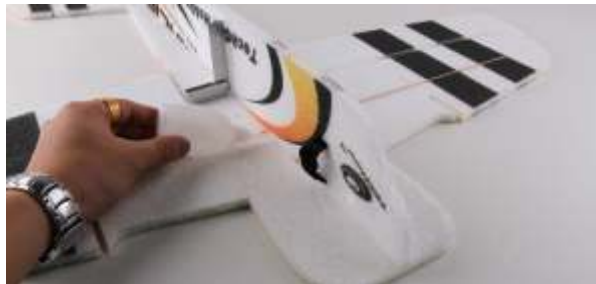
5. Install lower vertical fuselage on horizontal fuselage in place Make sure vertical fuselage is perpendicular to horizontal wing, then fix with glue.
