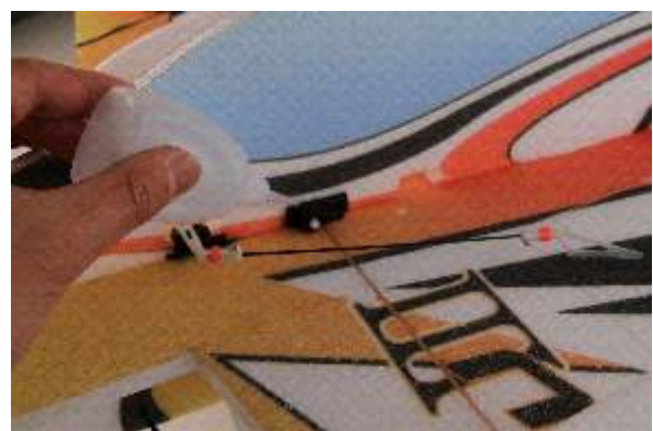
37. Put the servo in the slot of horizontal tail, then fix with glue
