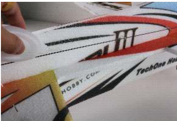
50. Install the fiber reinforcement in the slot of fuselage, make sure the reinforcement not be wiggly, then fix with glue
