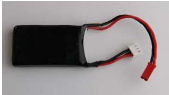
55.Battery: 2S 7.4V 400—500MAH
