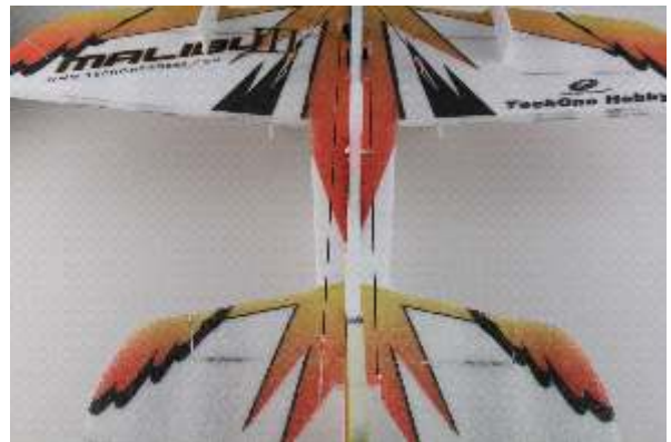
52. Rudder and elevator pushrods installation finished
