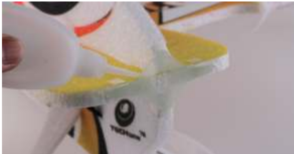
24. Put the motor mount on the nose of fuselage, then fix with glue
