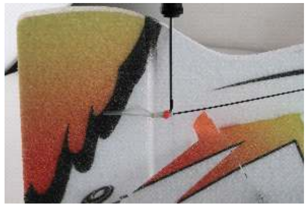
51. Adjust the plastic clip to the right place by screwdriver, then fix with screw
