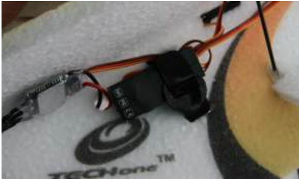
54.Connect and insert all servo cable to receiver according to suitable channel,then fix with velron ribbon
