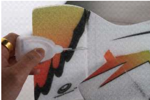
48. Install servo in the slot of rudder, then fix with glue
