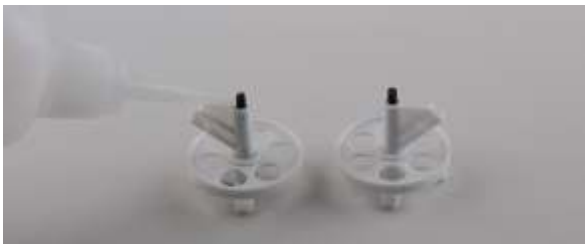
9. Then install wheel and triangle part, then fix axis and triangle part with glue
