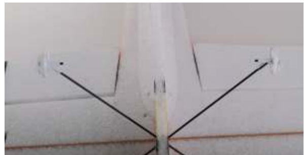
12. Place the U reinforcements on the joints of landing gear and lower fuselage, Make sure vertical fuselage is perpendicular to horizontal fuselage, then fix with glue.
