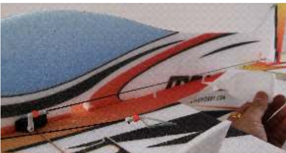
42. Install the fiber reinforcement in the slot of fuselage, make sure the reinforcement not be wiggly, then fix with glue.
