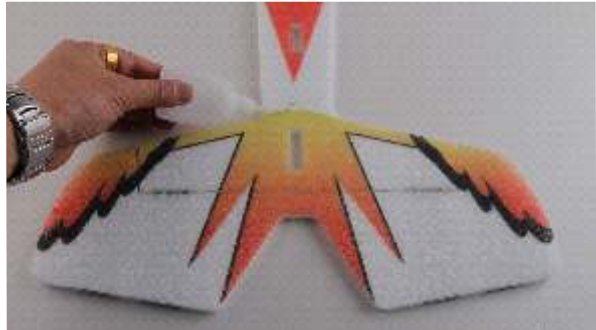
3. Horizontal stabilizer installation
