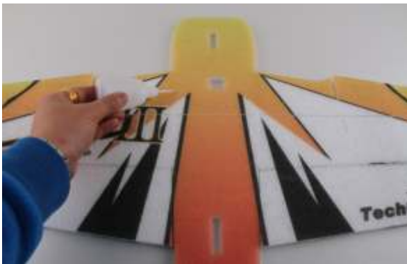
1. Glue left and right wing on fuselage as picture shown
