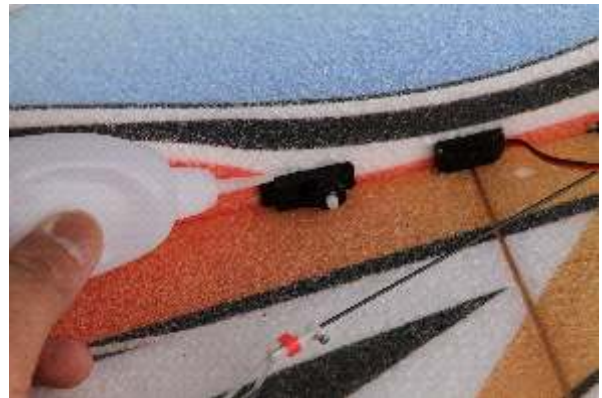
45. Install servo to the slot of rudder, then fix with glue
