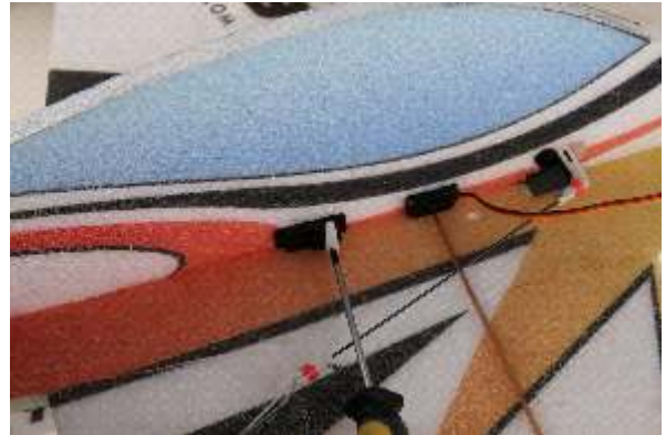
46. Install servo arm to servo, then fix with screw
