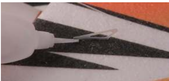
33. Put the control horn in the slot of left and right aileron, then fix with glue
