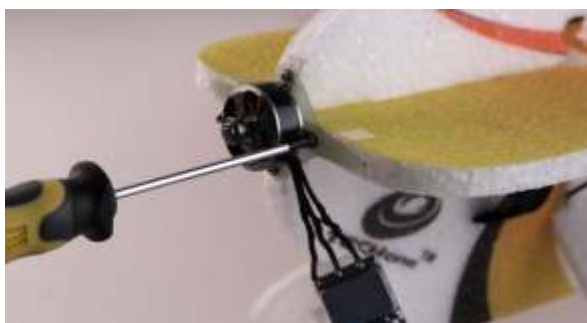
26. Fix the motor on motor mount with screw
