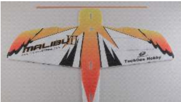
1. Glue left and right wing on fuselage as picture shown
