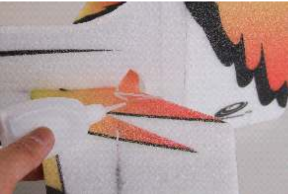
40. Put servo in the slot of horizontal tail, then fix with glue
