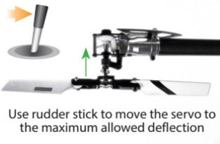
Use rudder stick to move the servo to the maximum allowed deflection
