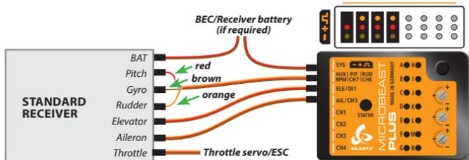
The illustrations are only intended as examples! The function assignment of the transmitter determines which channel on the receiver controls which function.
