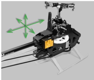
You can position MICROBEAST PLUS flat or upright on the helicopter. The large socket must point to the front or to the rear of the helicopter. The small white socket must be aligned with the longitudinal axis.
