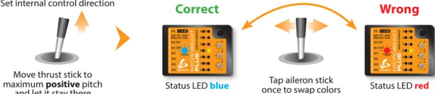
2. The Status LED must light solid, not just flash. If this is not the case, **increase the servo throw/endpoint of the pitch channel in the transmitter just as far so that the Status LED changes from flashing to solid when the rudder stick reaches the end position**. But do not increase the endpoint too much in the transmitter! We need an exact match of full stick position and stick end position, the Status LED should just change from flashing to solid when reaching the end position.
