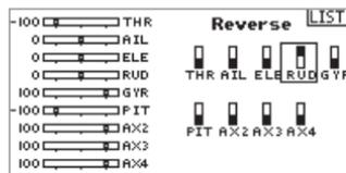
2. Now set the rudder direction of the MICROBEAST PLUS gyro
