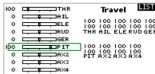
**⚠ With electric driven models remove the motor from the main gear when performing the basic setup for safety reason!** Additionally deactivate the throttle by using the „Throttle HOLD“ switch, so the motor won't start to turn when moving the thrust stick.
