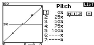
**Each control function must exactly control one output channel.** Initially the servo throws must be set to 100% and all trims and sub trims must be zero. For the basic setup do not change the pitch curves yet. The throttle curves and throttle servo settings can be adjusted as necessary for this model in case you do not intend to use the internal Headspeed Governor function of MICROBEAST PLUS.
