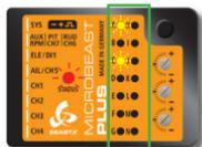
**This guide is intended to be used with MICROBEAST PLUS firmware version 5.0.x only!** After power up when the Status-LED lights red, for a few seconds in the left row menu LEDs **A** and **G** indicate major version „5“. In the right row no LED lights up.
