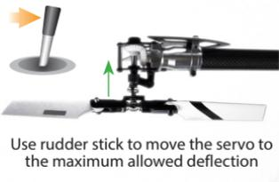
Use rudder stick to move the servo to the maximum allowed deflection
