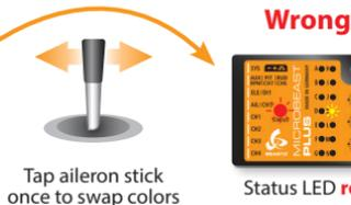
2. The Status LED must light solid, not just flash. If this is not the case, **increase the servo throw/endpoint of the pitch channel in the transmitter just as far so that the Status LED changes from flashing to solid when the rudder stick reaches the end position!** But do not increase the endpoint too much in the transmitter! We need an exact match of full stick position and stick end position, the Status LED should just change from flashing to solid when reaching the end position.
