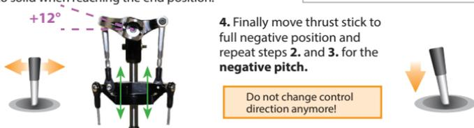
4. Finally move thrust stick to full negative position and repeat steps 2. and 3. for the **negative pitch**.
