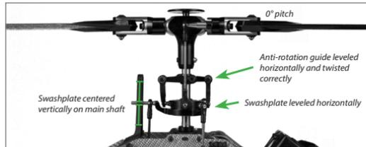
If necessary adjust the swashplate anti-rotation guide so that the swashplate phasing is not shifted (only applies to 2-blade rotorheads).
