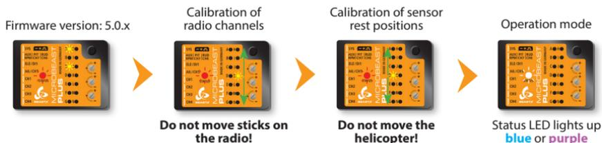
Then enter SETUP MENU for making the basic adjustments
