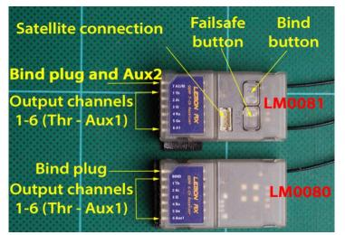
Both receivers have seven sets of pins on one end of the case: channels 1-6 are arranged in the usual Spektrum order of T, A, E, R, G, Aux1.
