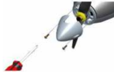
13. Install the spinner, then fix with screw.
