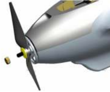
12. Put on the washer and nut, then screw down.
