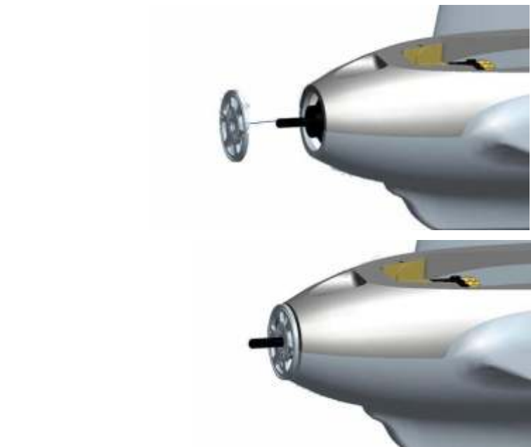
9. Place spinner backboard on motor shaft.
