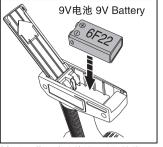
Remove the battery cover on the controller, place 1 x 9V battery into the battery compartment with correct polarity.
